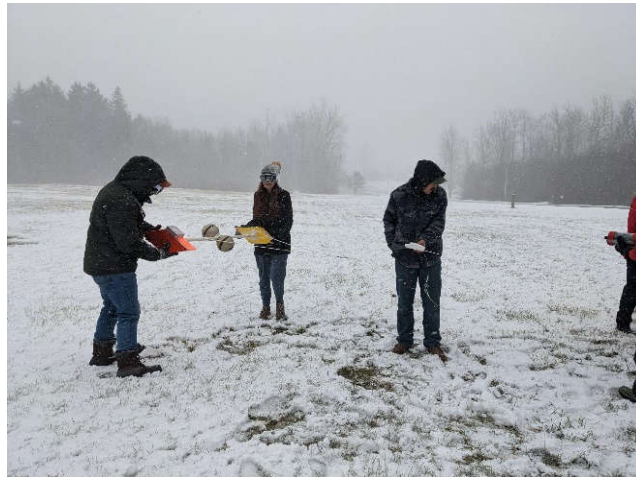
Figure 1. Electric field meter (left) with radiosonde (middle) and cutdown/letdown package (right) ready to launch in LEE.
